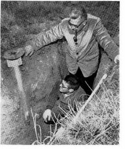
MAN, DIG that crazy postholer! Penetrometers designed and developed by Terradynamics 9327 make a nice, neat hole in the ground but serve a more useful function as a means to obtain remotely the soil data necessary to establish airfields in forward or hostile areas. John Colp (standing) and Ed Villella (both 9327), examine one of the earth penetrating instruments after test drops made at Sandia recently.
